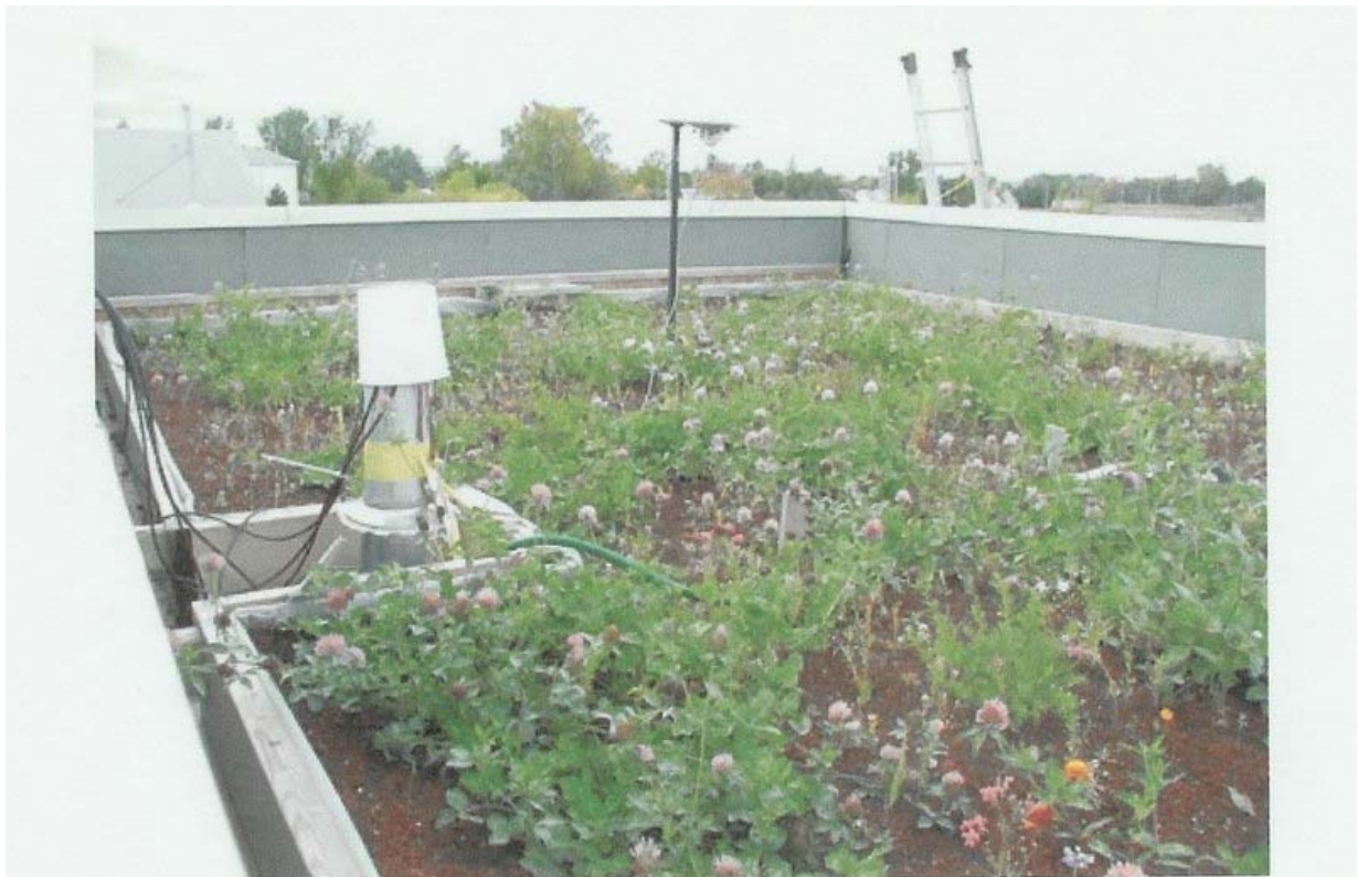
Photo courtesy of the National Research Council Canada, Ottawa. A green roof system was built on the Field Roofing Facility at the National Research Council Canada's campus in Ottawa. The wildflowers growing on the green roof system are native to Ontario or adapted to its climate.
